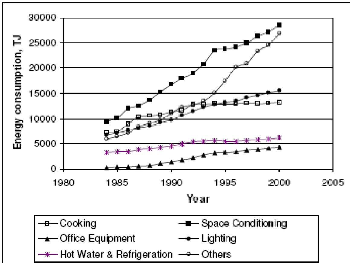
Figure 4 – Energy end-uses of the commercial sector of Hong Kong in 1984 to 2000
